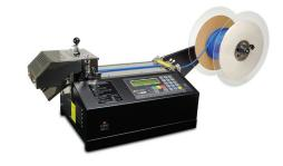
Ideal for cutting insulating sleeves, sleeving, Nomex®, etc. This machine is fully controlled by a microprocessor and using a stepping machine guarantees maximum precision in executing tasks. It is fitted with a safety device that automatically stops the cut if the material comes out. It does not require further blades for the various materials to be cut.
