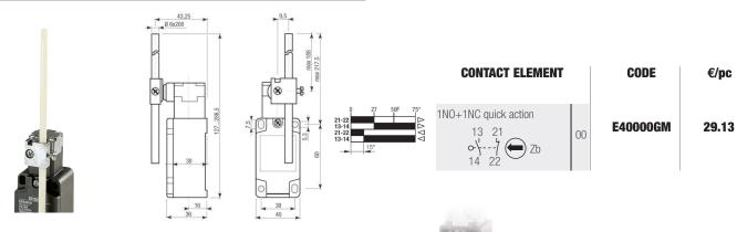
4 holes for fastening with 30 mm horizontal distance between centres and adjustment slots. Compliant with standards IEC/EN 60947-1 IEC/EN 60947-5-1
